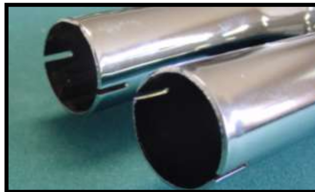
Above - Slotted End of Tip (inlet)
