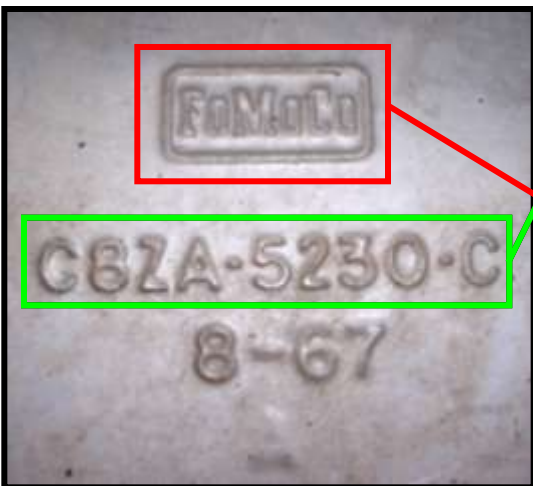
Above - Original 1968 Muffler Stamping
