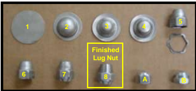
Above - New Lug Nut Fabrication Sequence
