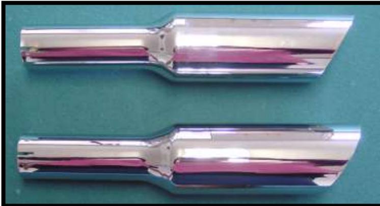
Above - Original NOS Tip (top) & New Reproduction (bottom)
